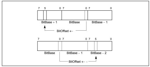
Figure 3-2. Memory Bit Indexing
