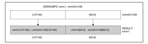
Figure 3-3. ADDSUBPD: Packed Double-FP Add/Subtract
